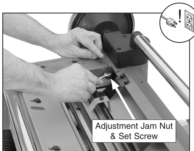
Figure 66. Example of adjusting the pressure bar height.
