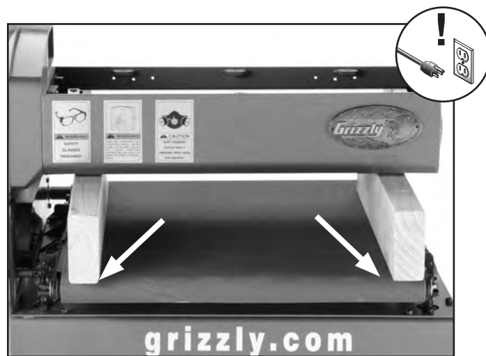
Figure 47. Example of gauge blocks placed under drums.
