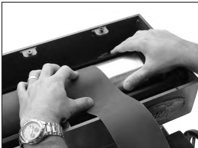
Figure 20. Wrapping sandpaper around drum.
