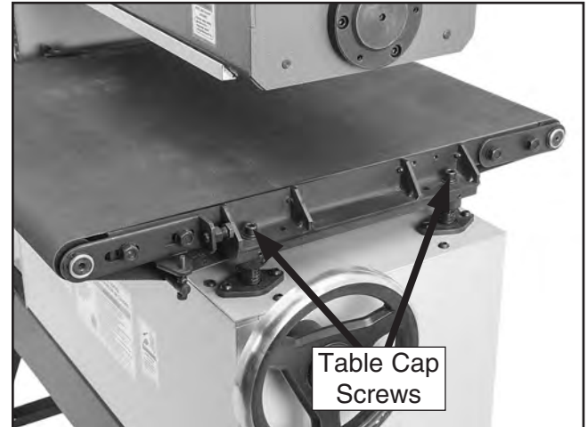
Figure 41. Feed belt table outside cap screws.
