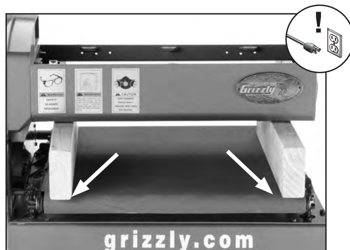
Figure 45. Example of gauge blocks placed under drum.
