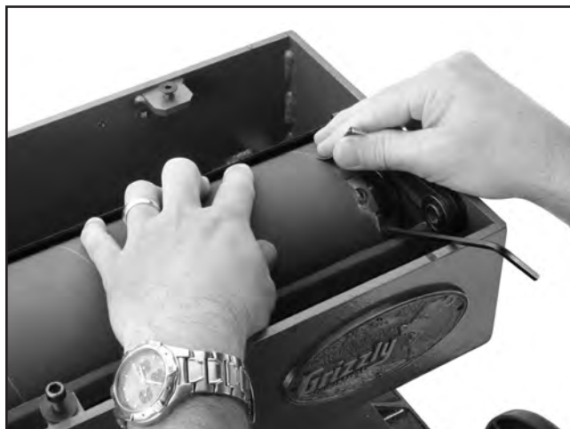
Figure 22. Wrapping sandpaper over tension wheel.
