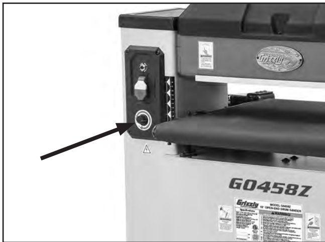
Figure 16. Location of conveyor feed rate dial.
