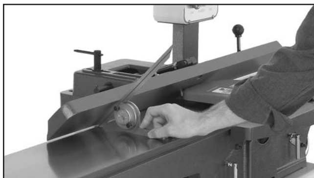
Figure 50. Example of adjusting fence 45° inward.
