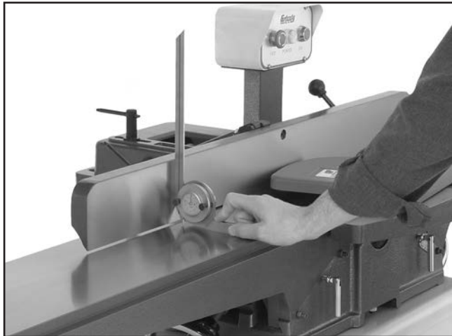
Figure 52. Adjusting fence to 90°.
