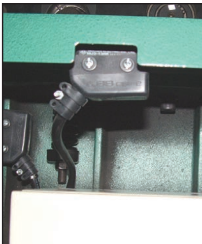
Figure 53. Headstock cover limit switch (top right access panel removed).
