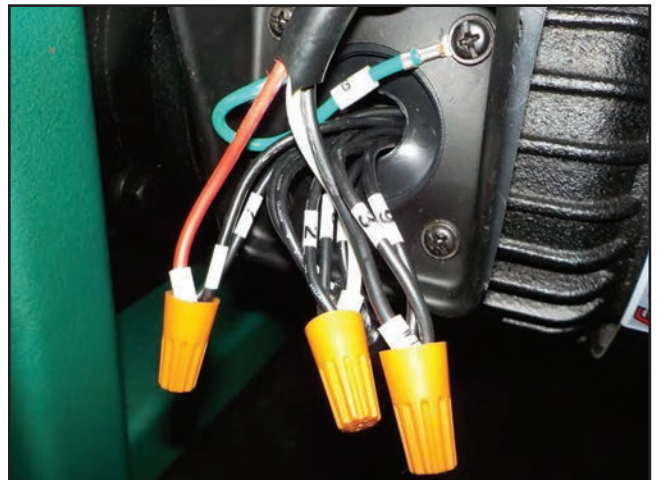
Figure 55. Table motor junction box wiring.
