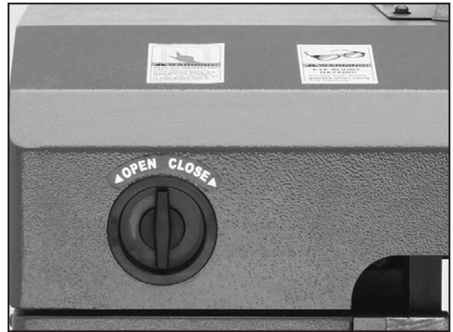
Figure 19. Headstock cover latch in closed position.
