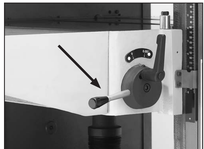
Figure 22. Table roller height control.
