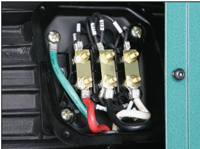
Figure 52. Cutterhead/feed motor junction box.
