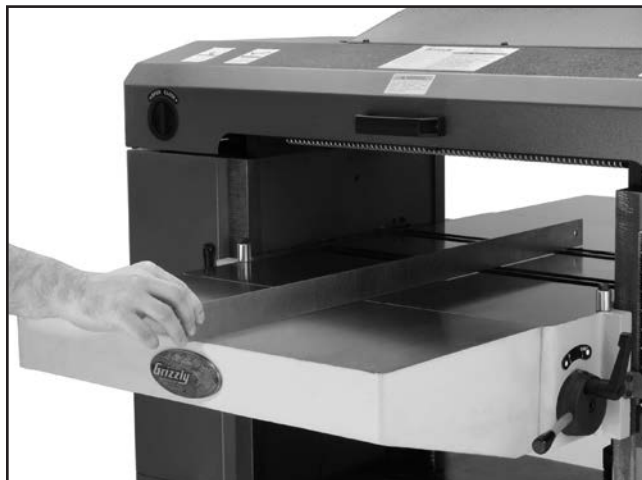
Figure 14. Leveling extension wings and table.
