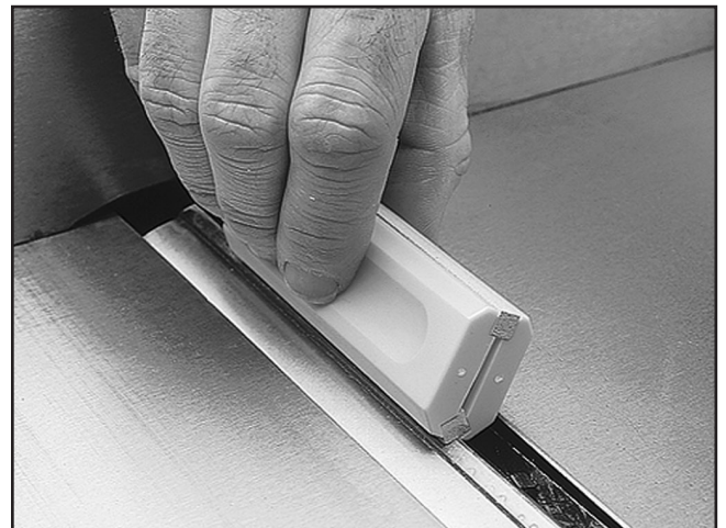
Figure 37. G3631 Jointer/Planer Knife Hone.
