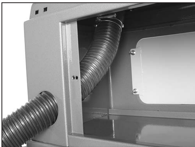
Figure 17. Dust hose attached to dust port.
