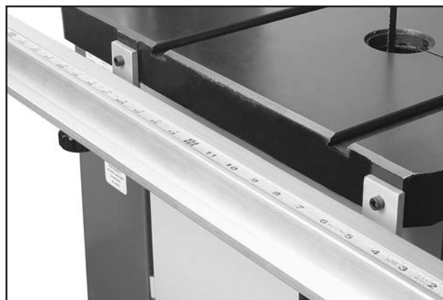
Figure 15. Scale installed on front fence rail.
