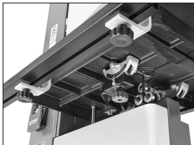
Figure 10. Fastening front fence rail.
