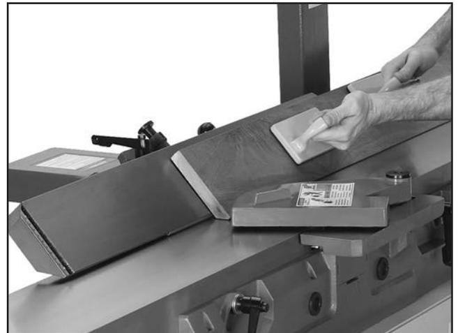
**Figure 30.** Typical bevel cutting operation, fence stop at  $45^\circ$  outward.
