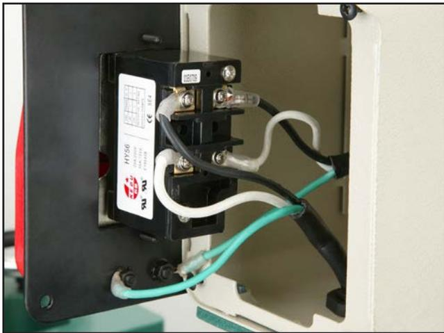
Figure 65. Switch wiring.
