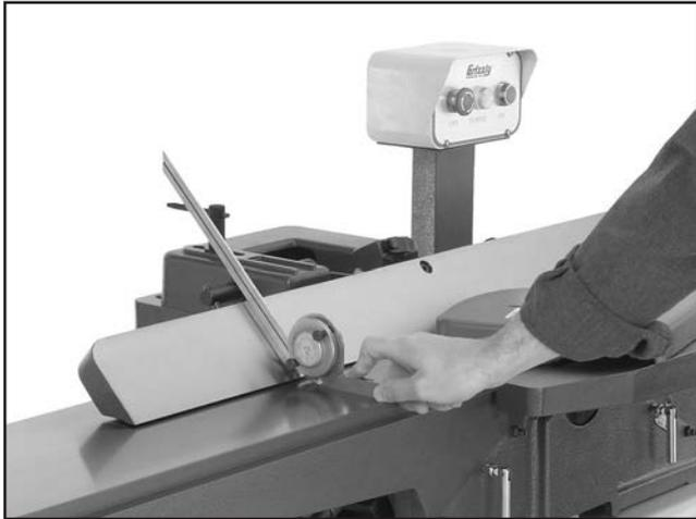
**Figure 62.** Example of adjusting fence 45° outward.
