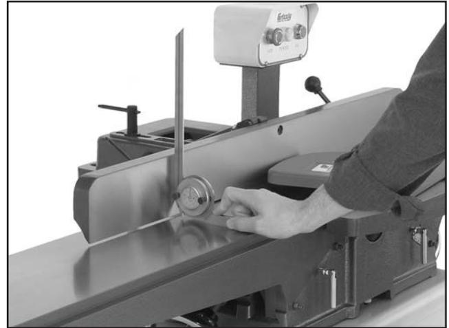
**Figure 60.** Example of adjusting fence to 90°.
