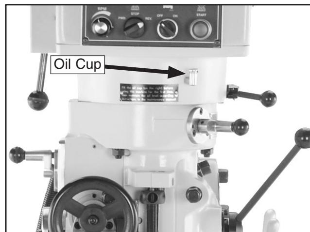
**Figure 52.** Speed range gearing oil cup.
