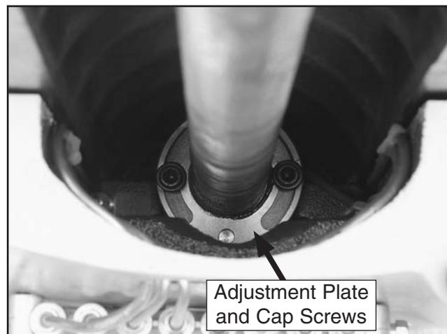
**Figure 69.** Longitudinal leadscrew adjustment plate and cap screws as seen from the left underside of the table.
