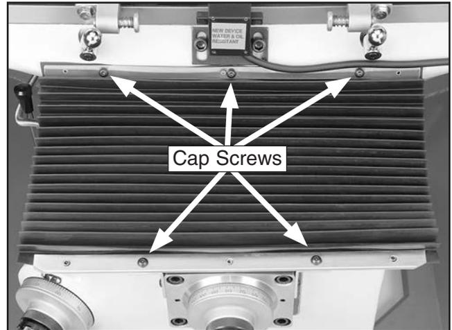
**Figure 13.** Front way cover installed.
