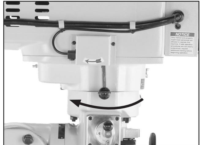
**Figure 39.** Emergency spindle brake on the left side of the head.
