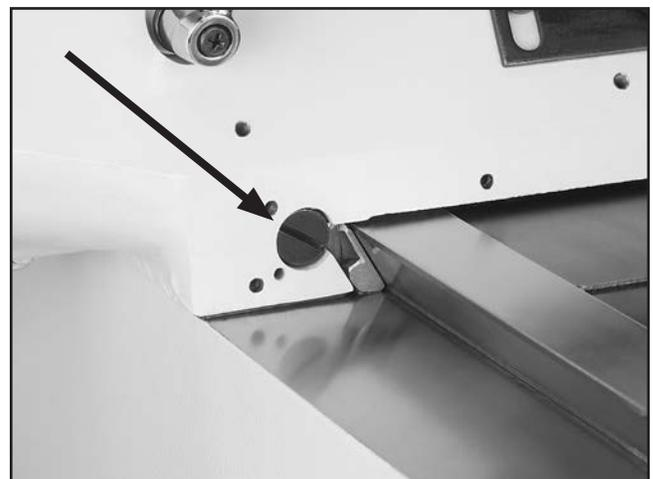
**Figure 63.** Saddle gib adjustment screw (front adjustment screw shown).
