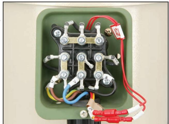
Figure 75. Spindle motor wiring.
