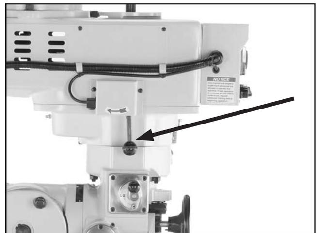
Figure 19. Emergency spindle brake.
