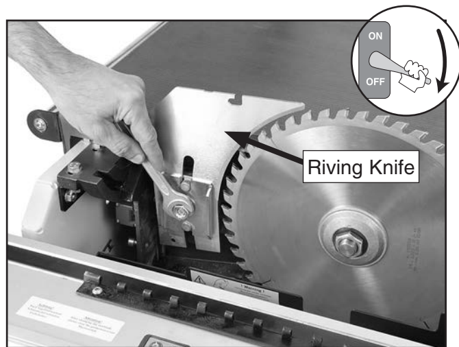
Figure 55. Re-adjusting the riving knife.
