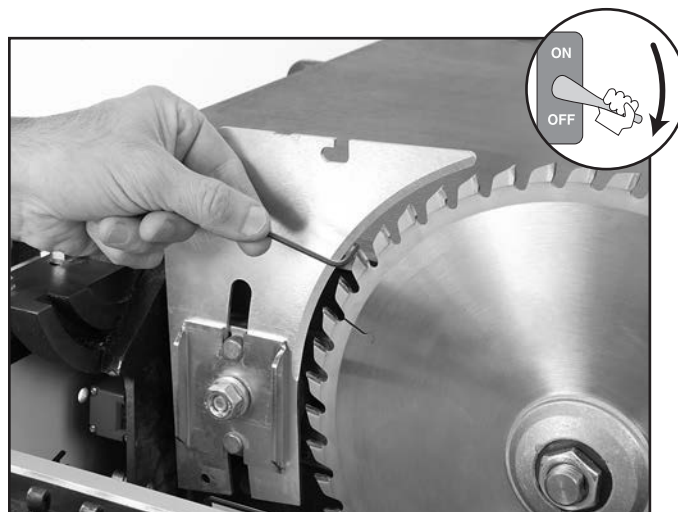
Figure 56. Aligning the riving knife.
