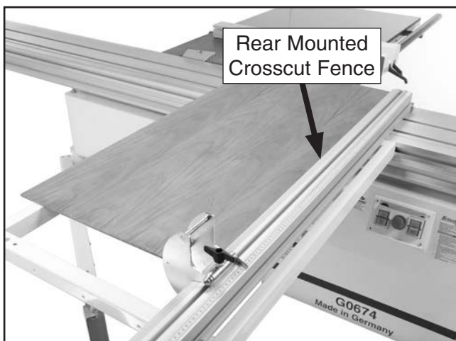
Figure 69. Crosscutting smaller panels.
