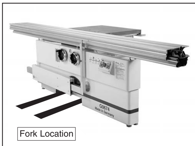
Figure 11. Lifting the saw base unit.
