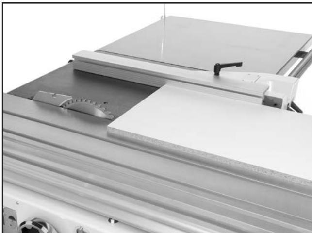
Figure 62. Traditional rip cutting.
