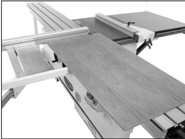
Figure 61. Rip cutting with the sliding table.
