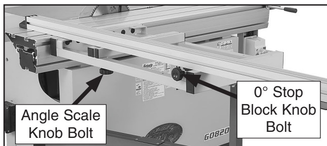
Figure 160. Locations of knob bolts securing crosscut fence.
