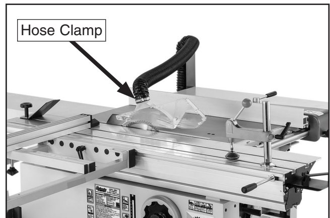
Figure 56. Blade guard and 2½" dust hose attached.
