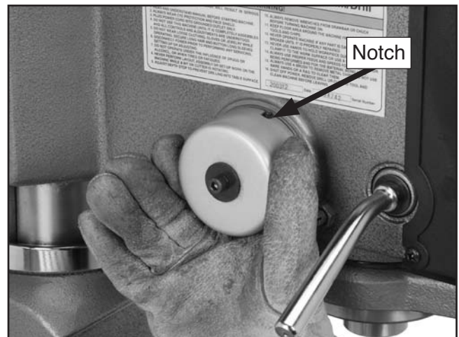
Figure 44. Adjusting spring tension.
