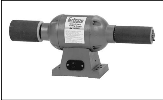
Figure 3. Sanding drums installed.
