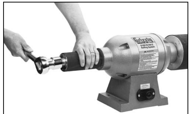
Figure 5. Sanding drum loosening/tightening procedure.
