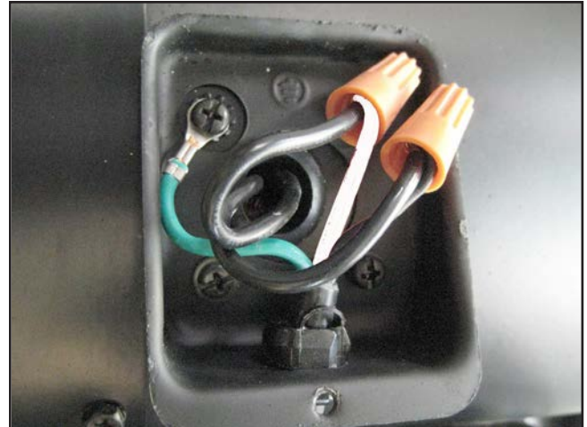
Figure 68. G1079R drum motor connections.
