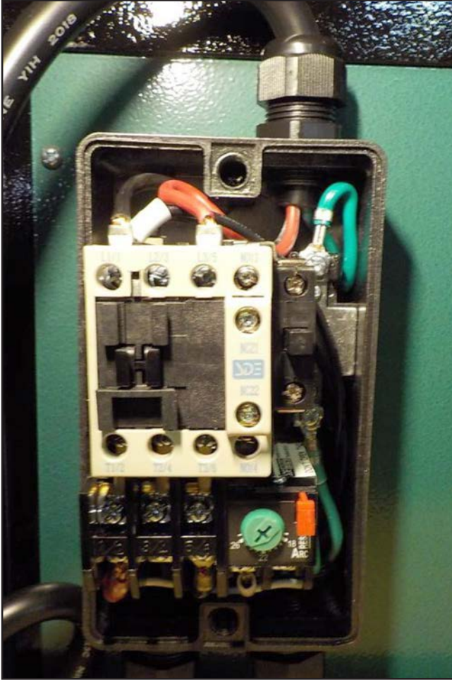
Figure 59. G1066R magnetic switch connections.
