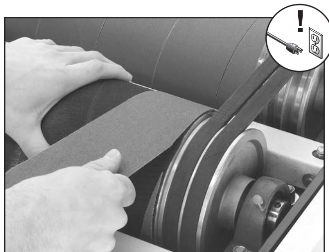
Figure 29. Example of wrapping sandpaper around drum.
