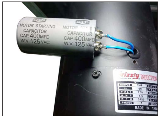
Figure 69. G1079R drum motor start capacitor.
