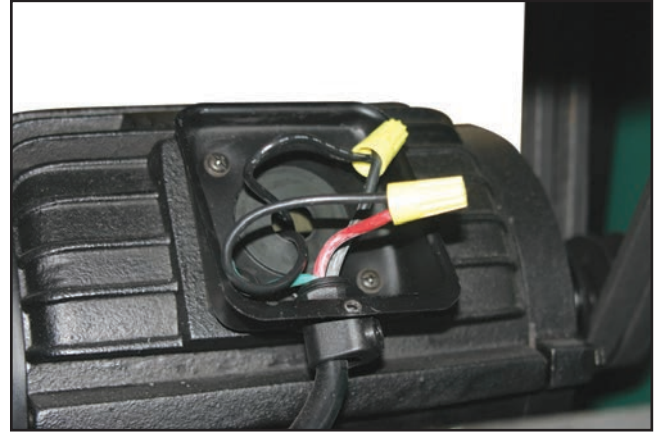
Figure 61. G1066R drum motor connections.
