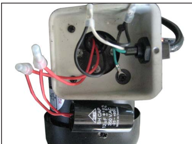
Figure 67. G1079R feed motor connections and run capacitor.
