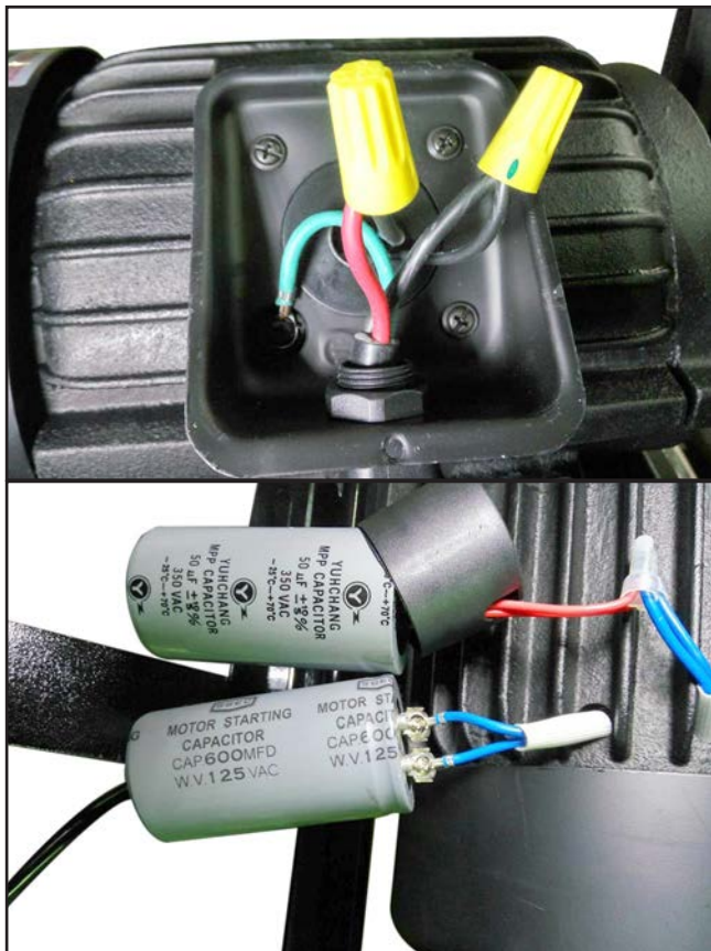
Figure 63. G1066Z drum motor connections and capacitors.
