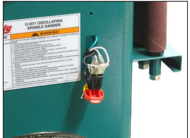
Figure 38. Switch wiring.
