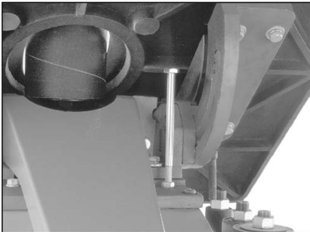
**Figure 12.** Table stop bolt (table tilted for clarity).
