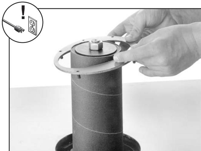
**Figure 24.** Installing table insert.
