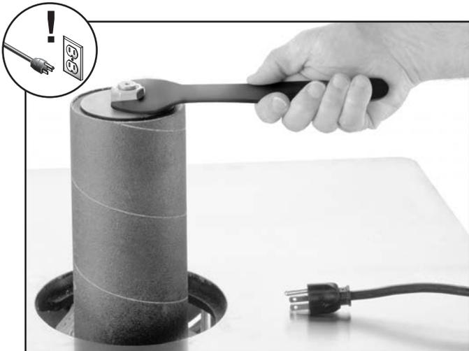
**Figure 22.** Removing sanding sleeve.
