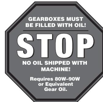
It is critical that you make sure there is oil in the gearbox before proceeding with the test run. Remove the spindle gearbox oil fill cap and use the dipstick to make sure the oil level is full. When full, the oil will read on the knurled portion of the dipstick.
