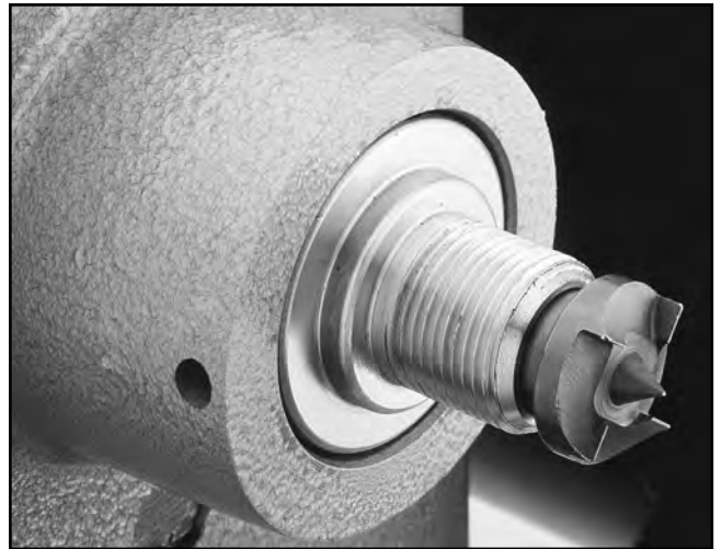
Figure 15. Spur center in headstock spindle.
