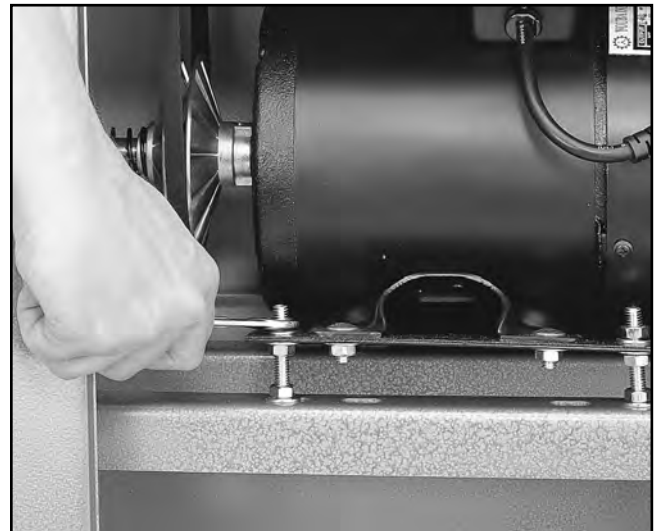
Figure 7. Loosening motor mount bolts.
