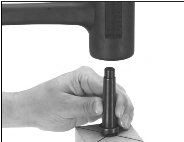
Figure 25. Seating the spur center.
