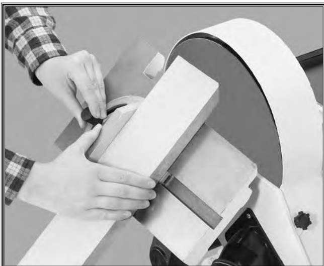
Figure 37. Using table to sand angles.
