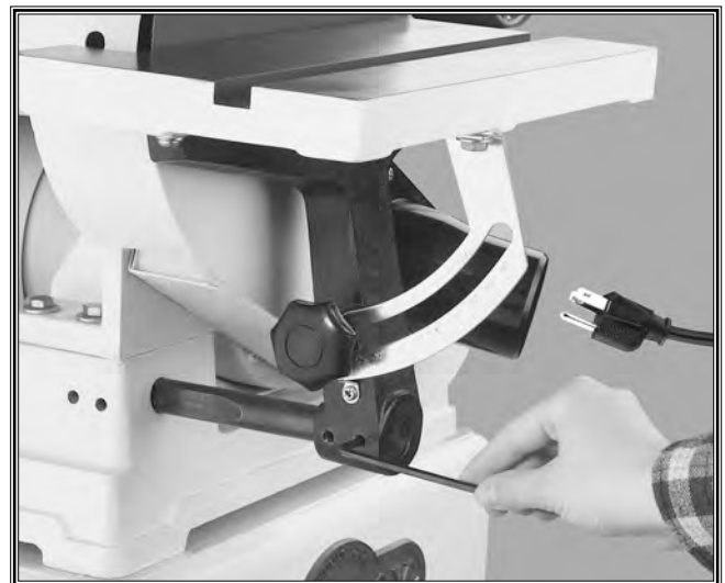
Figure 16. Tightening the setscrews.
