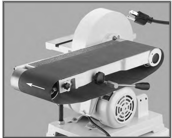
Figure 18. Installing the sanding belt.
