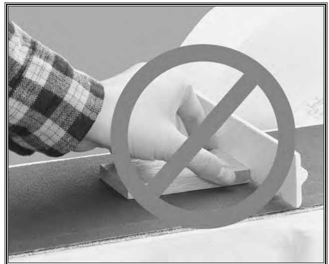
Figure 6. Never place hands near back stop. On small workpieces always use push blocks.
