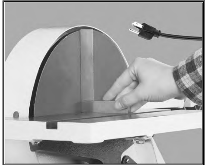
Figure 29. Checking table alignment.
