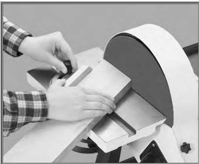
Figure 36. Using miter gauge to sand angles.
