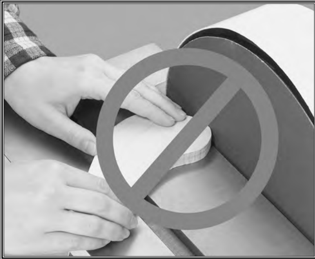
Figure 3. Never place fingers close to moving disk.
