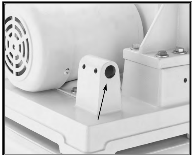
Figure 25. Working table mounting hole when vertical sanding.
