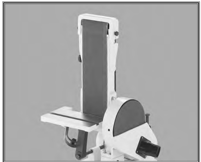
Figure 24. Belt sander in vertical position.
