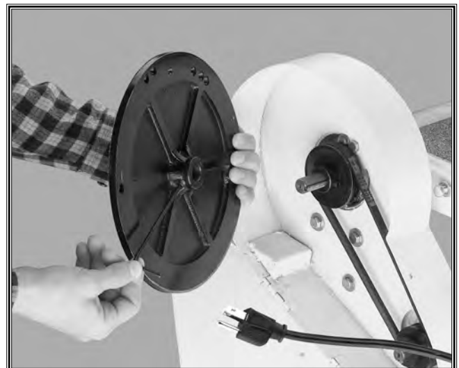
Figure 11. Installing sanding disk.
