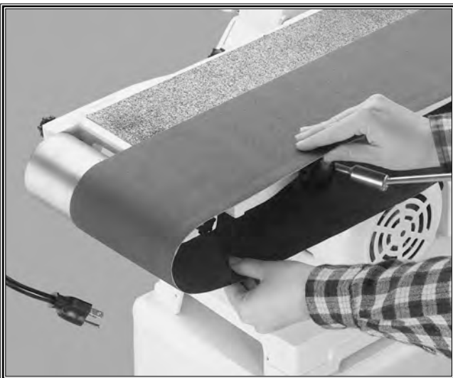
Figure 5. Always unplug sander when adjusting.
