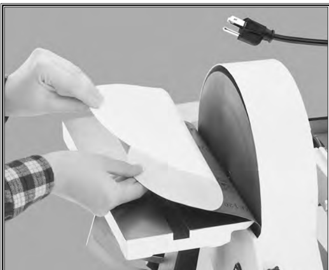
Figure 28. Changing abrasive disc with table on.
