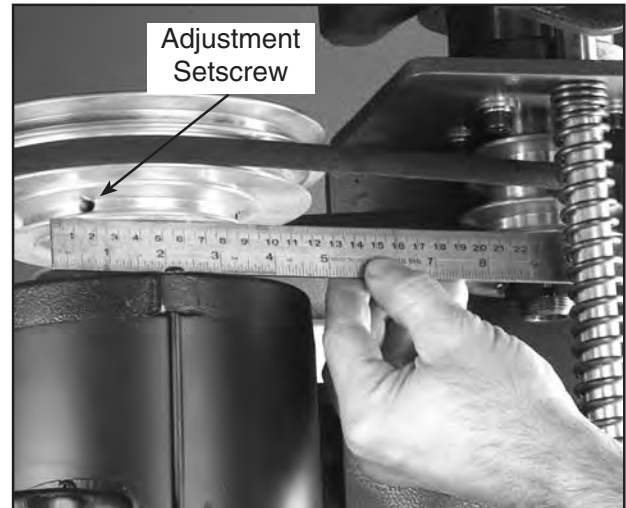
Figure 22. Inspecting pulley alignment.
