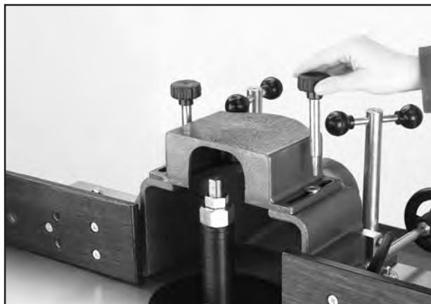
Figure 18. Installing guard cover.
