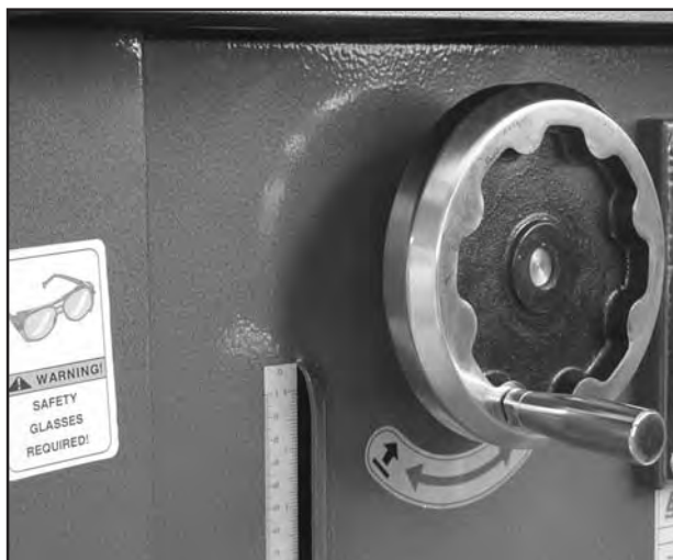
Figure 19. Handwheel mounted to shaper.
