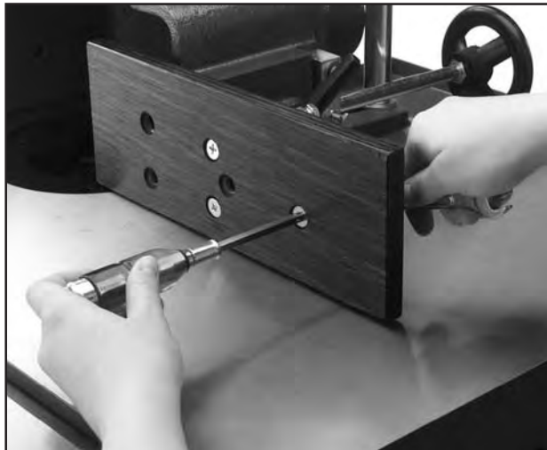
Figure 17. Attach wooden fence assembly.
