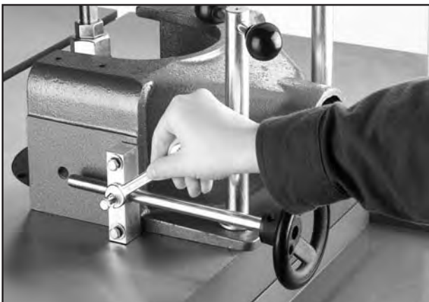
Figure 14. Tightening bolt into shaft groove.
