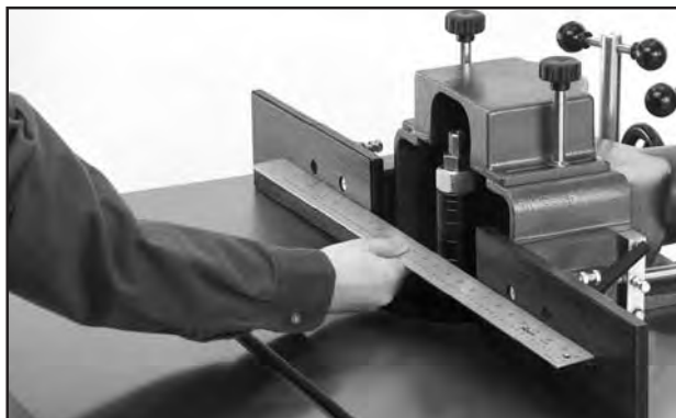
Figure 25. Aligning fences with straightedge.
