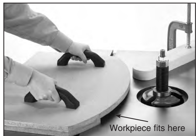
Figure 39. Pattern jig for making curved pieces.
