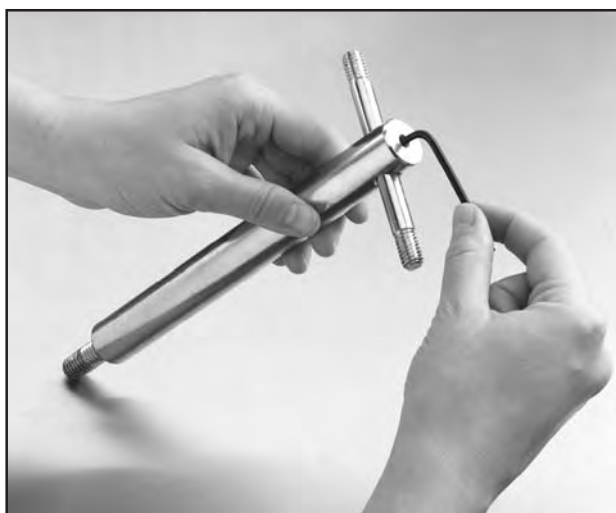
Figure 10. Tightening setscrew with hex key.
