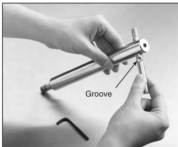
Figure 9. Bar into shaft guide.
