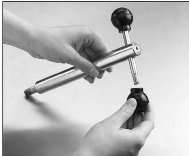
Figure 11. Round knobs onto bar.
