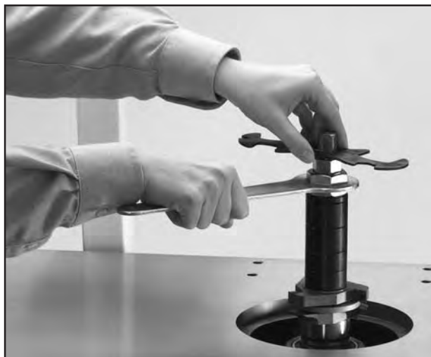
Figure 29. Tightening spindle nuts.
