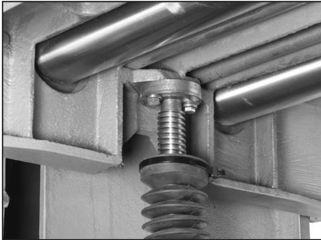
Figure 14. Column adjustment flange underneath table.
