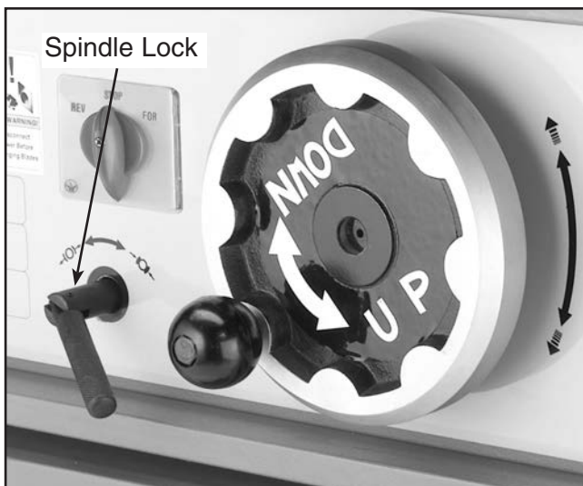
Figure 19. Spindle height adjustment wheel and spindle lock.
