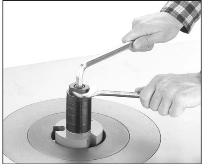
Figure 15. Tightening spindle nuts.
