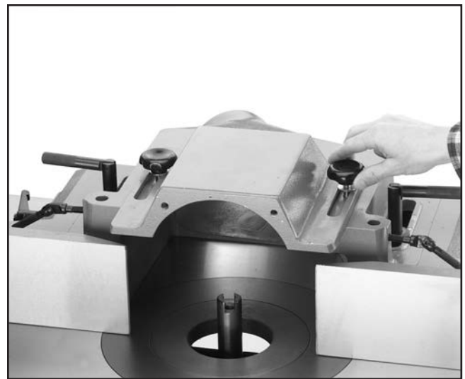
Figure 6. Installing the cutter guard.
