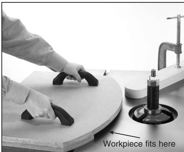
Figure 29. Pattern jig for making curved pieces (guard removed for clarity).
