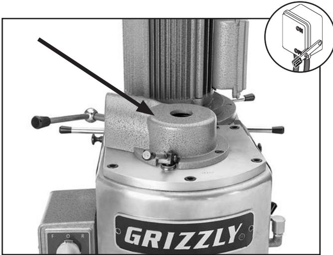
**Figure 58.** Model G9901/G9902 drawbar access.
