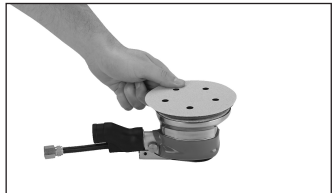
Figure 2. Attaching sanding disc.
