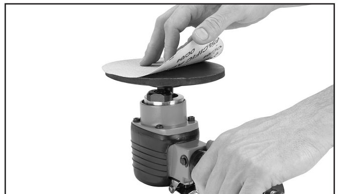
Figure 3. Attaching sanding disc.
