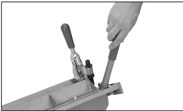
Figure 5. Breaker bar lever installation.
