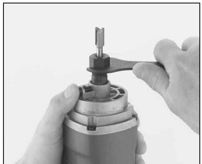
Figure 5. Tightening bit into router.
