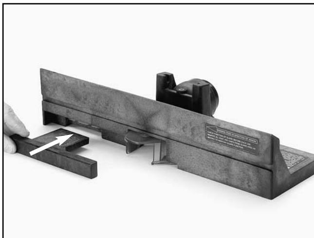
Figure 13. Installing the pocket jointing fence.
