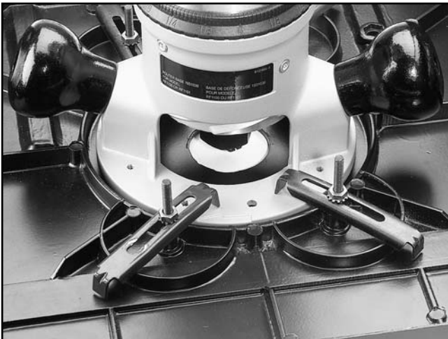
Figure 10. Correctly clamped router.
