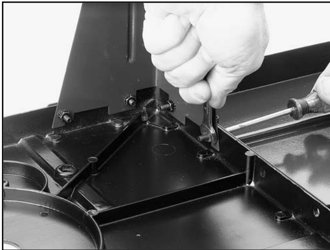
Figure 5. Securing a leg to the main table.
