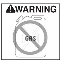
Gasoline or petroleum products used to clean the tool could explode causing serious personal injury. DO NOT use gasoline or petroleum products to clean the tool.
