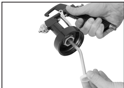
Figure 4. Installing H3254 filter.
