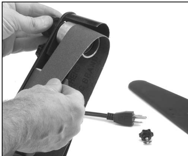
Figure 19. Removing sanding belt.
