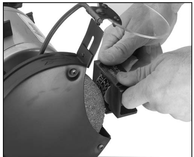
Figure 11. Using wheel dressing tool.
