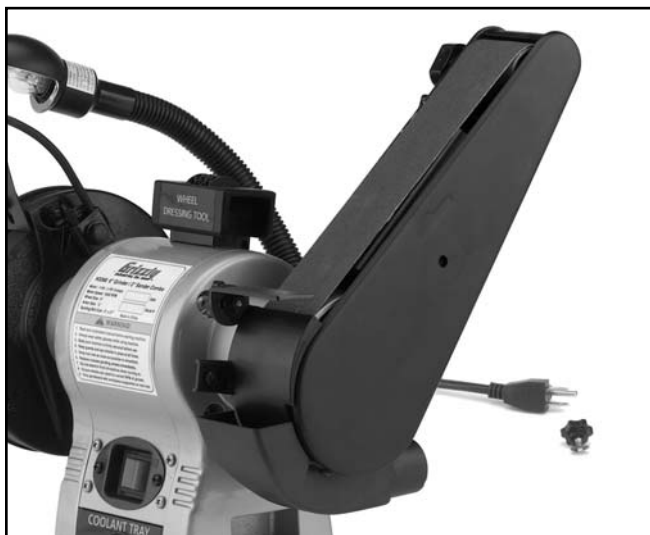
Figure 17. Removing star knob from cover.
