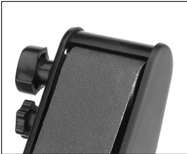
Figure 9. Sanding belt centered between belt cover edges at the upper roller.
