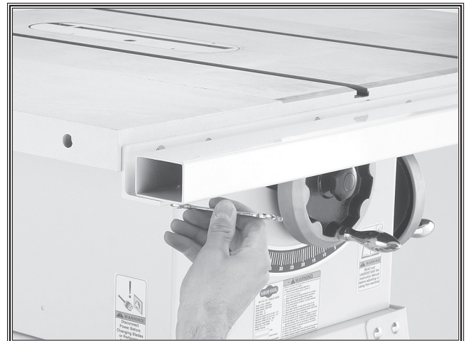
Figure 4. Installing fence tubing.
