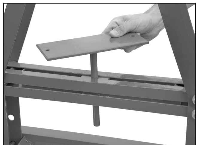
Figure 6. Jack plate installation.
