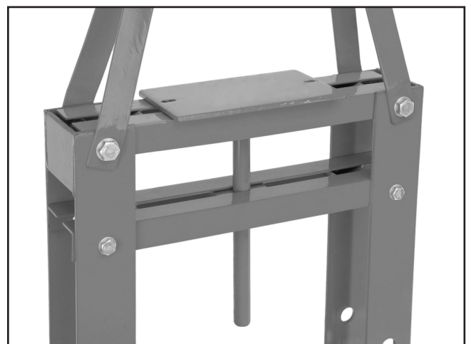
Figure 6. Jack plate installation.
