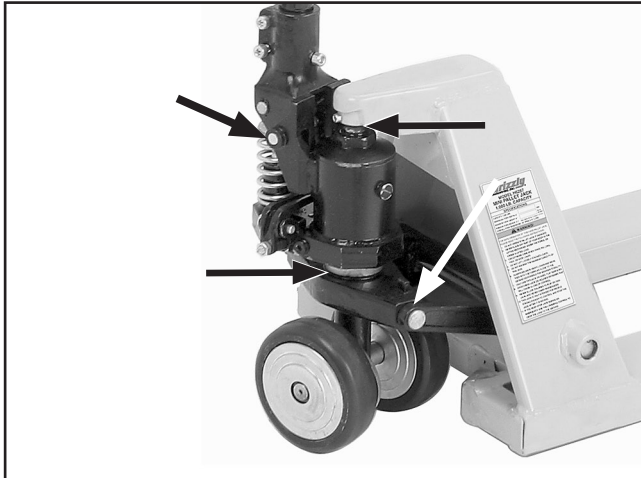
Figure 13. Lubrication locations, Model H6287/H6288.
