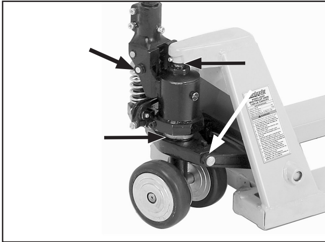
Figure 13. Lubrication locations, Model H6287/H6288.
