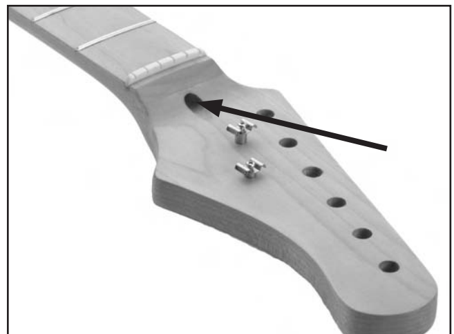
Figure 26. Truss rod nut location.
