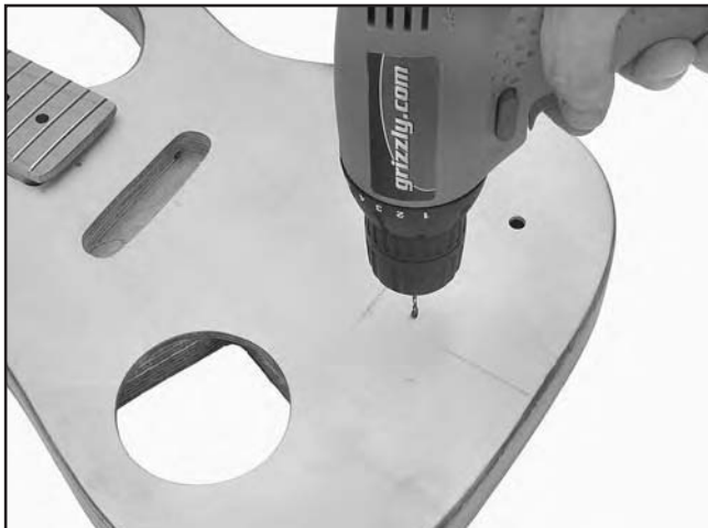
Figure 6. Drilling ground wire pilot hole.
