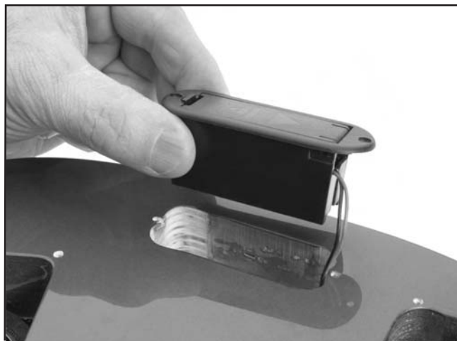
Figure 13. Installing battery case.
