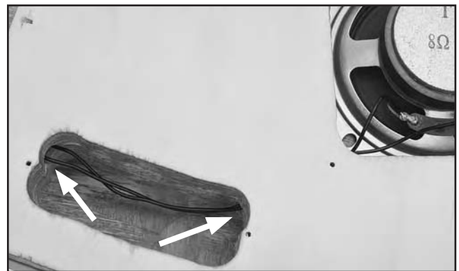
Figure 11. Speaker wires in battery case mortise.
