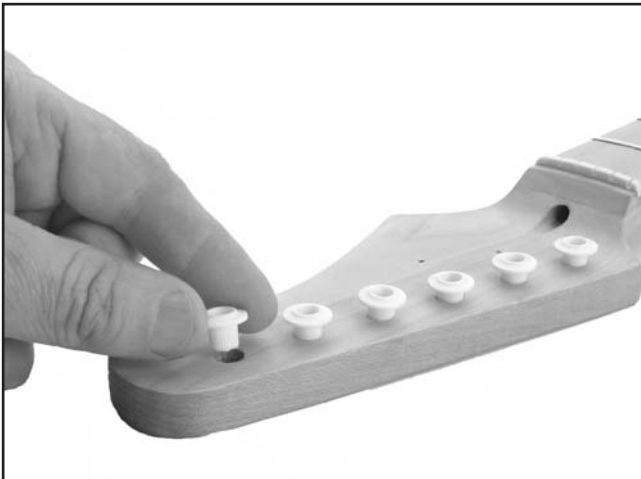
Figure 6. Installing plastic bushings on headstock.
