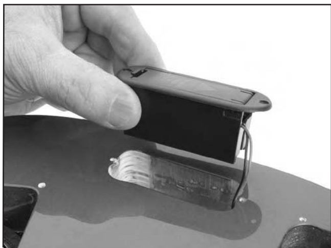
Figure 12. Installing battery case.
