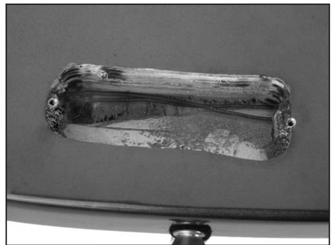
Figure 12. Speaker wires in battery case mortise.
