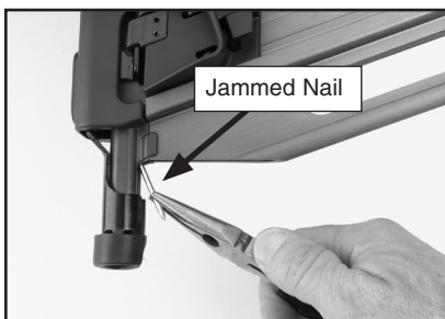
Figure 11. Using pliers to remove a jammed nail.
