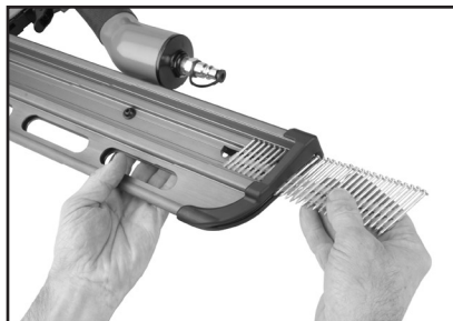
Figure 3. Loading nails in the magazine.
