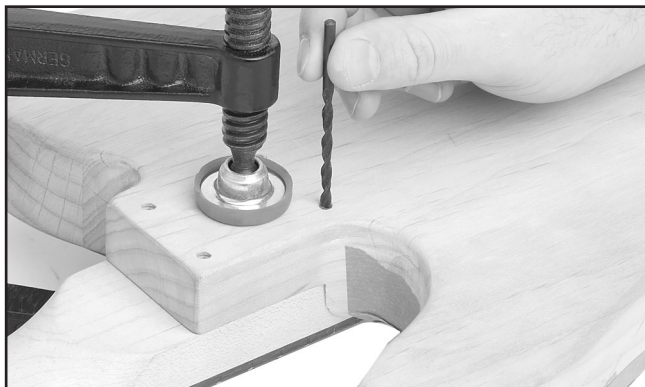
Figure 10. Example of making a pilot hole in the neck.
