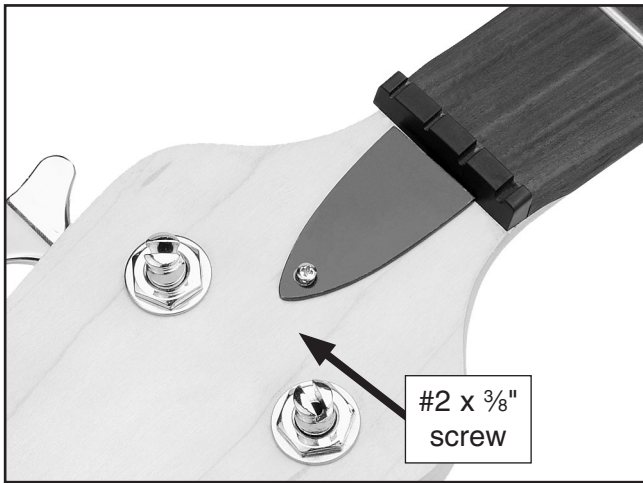
Figure 26. Truss rod cover installed.
