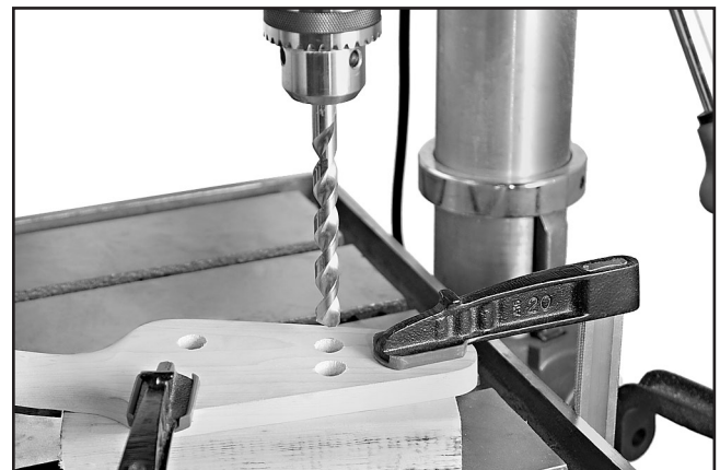
Figure 7. Drilling the pegholes.
