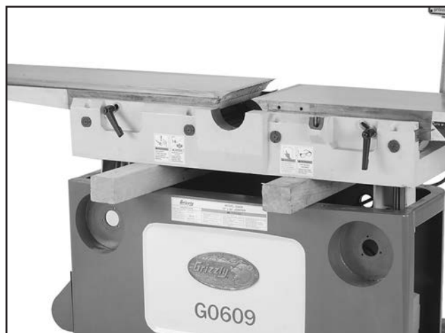
Figure 8. Jointer bed supported with 4x4s on both ends.
