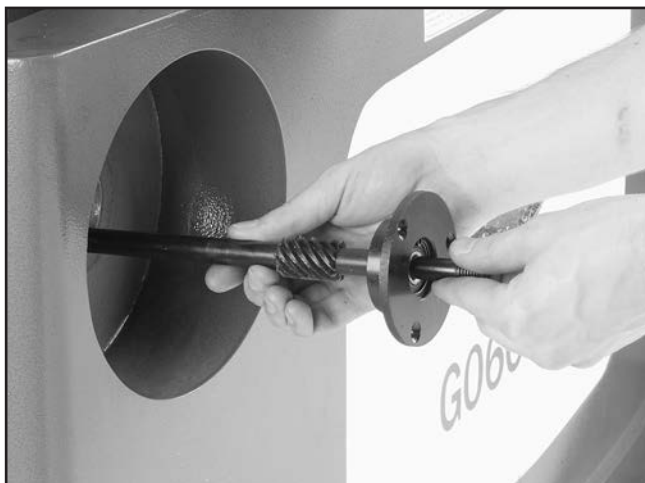
Figure 6. Removing spiral gear shaft.
