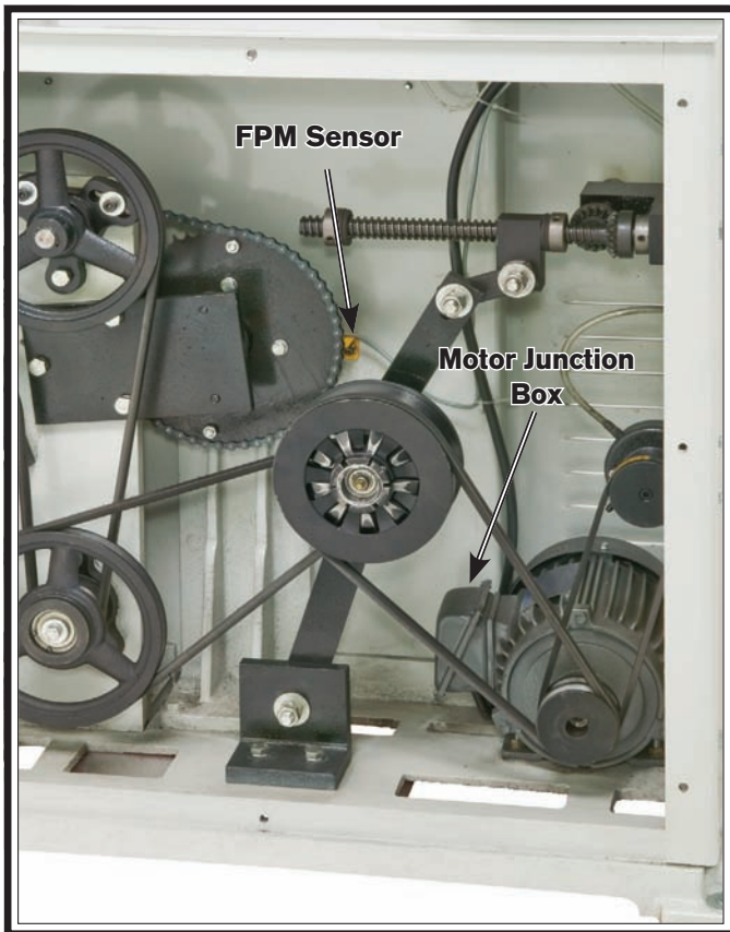
Figure 53. Motor and FPM sensor.
