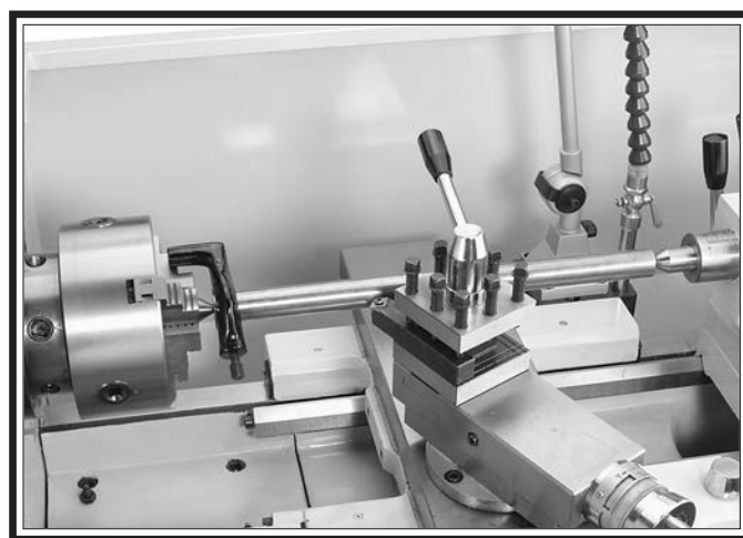
Figure 52. Example photo of a workpiece mounted between the centers.
