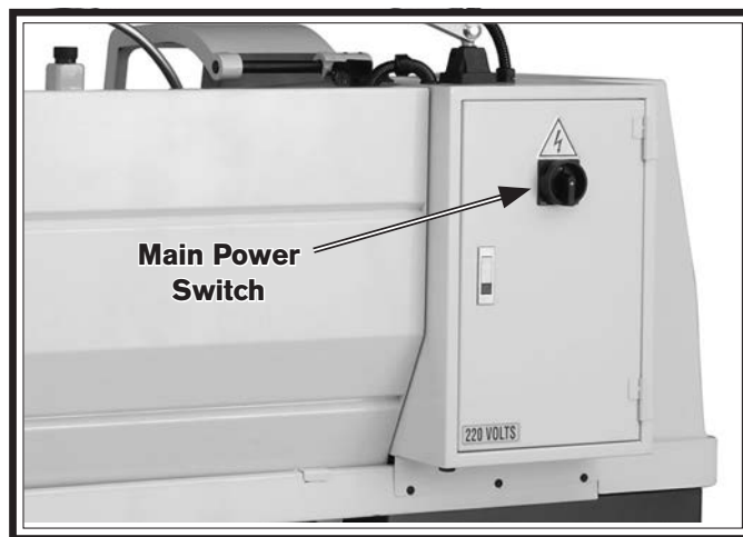
Figure 22. Location of the master power switch.
