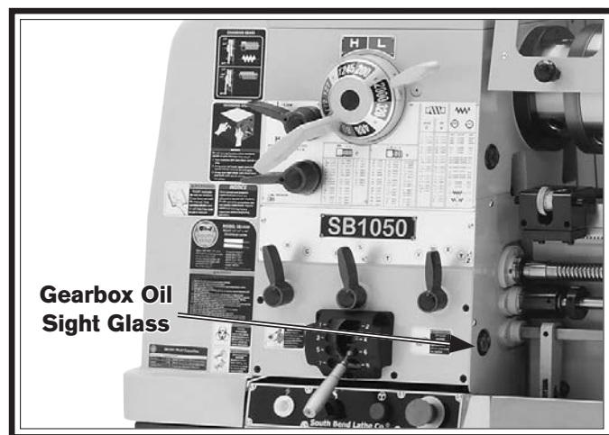
Figure 101. Location of quick-change gearbox oil sight glass.
