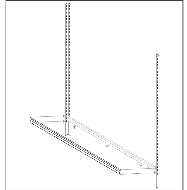
Figure 2. Attaching long shelf support.
