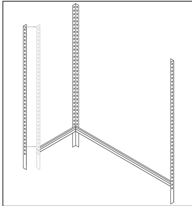
**Figure 4.** Attaching a third rail.
