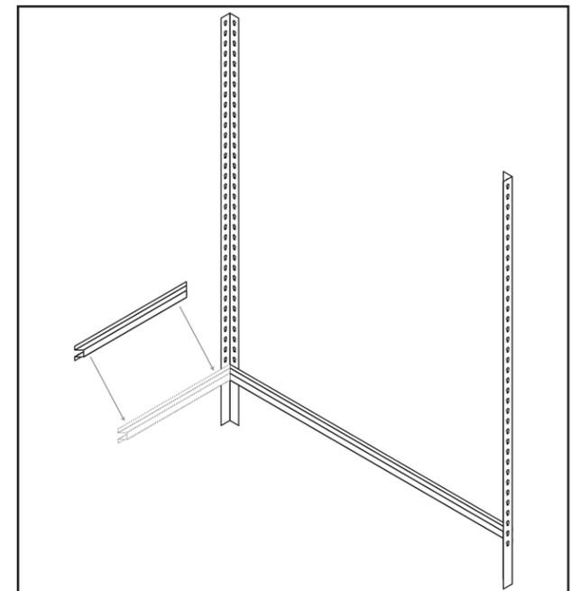
Figure 3. Attaching short shelf support.
