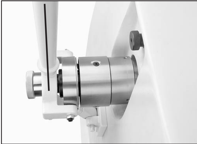
Figure 13. Unlocked collet-closer lever.
