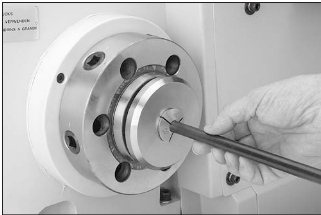
Figure 9. Installing a workpiece.
