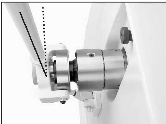
Figure 14. Locked collet-closer lever.
