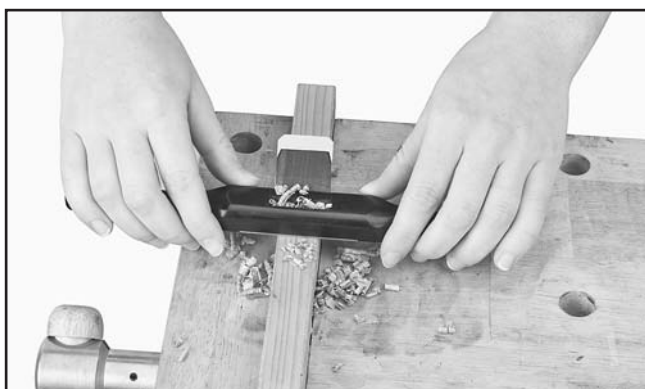
Figure 4. Example of pushing the spokeshave.
