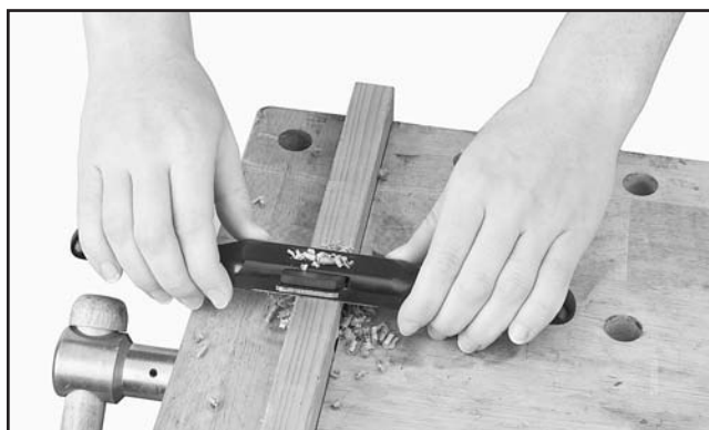
Figure 5. Example of pulling the spokeshave.
