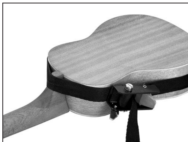
Figure 4. Securing the ukulele neck to the body.
