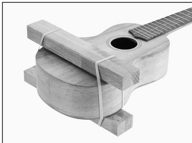
Figure 12. Gluing the bridge to the body.
