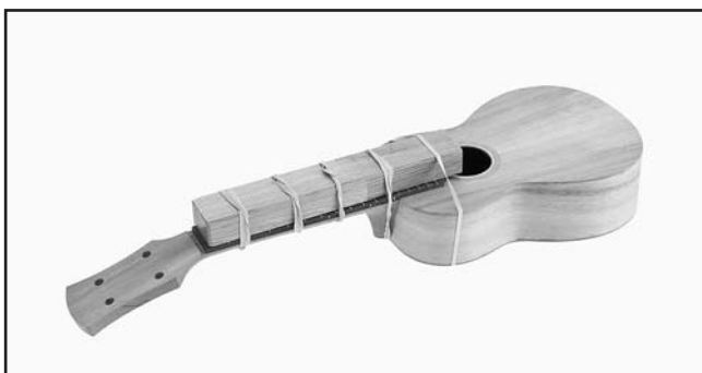
Figure 6. Attaching fingerboard to the neck.
