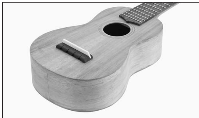
Figure 13. Bridge and saddle installed on the sound board.
