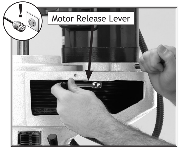
Figure 29. Releasing tension to V-belt.
