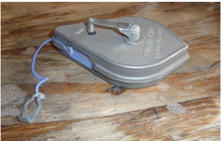
Chalk line used to set center reference line.
