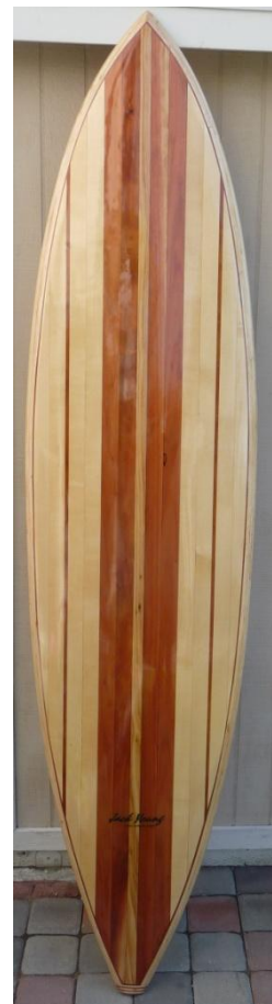
This is the new semi gun shape with the rails installed.
