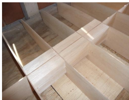
As a minimum 1½” wide balsa (or other light wood) blocks are needed for the mast box mount.
