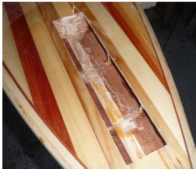
The ribs and spar are cut and removed and the area is cleaned of debris.
