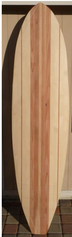
This is the how the 7' 6" egg looks before the rails are installed.
