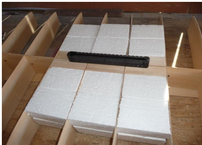
The mast box and fin box are installed after the board is glassed as described in chapter 12 of this book.
