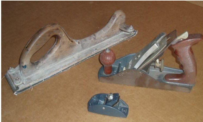
Hand planes and a long board sanding block. Using a hand plane creates much less mess than a belt sander.
