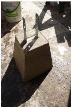
Build a shaping stand using a cement foundation pier for a base (about $6.00 at Home Depot). You can store it away when not in use.
