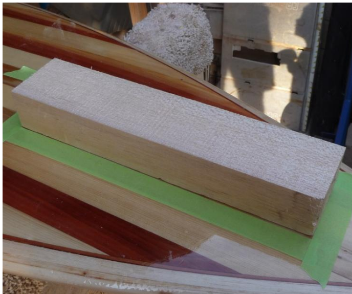
A solid balsa block is cut to size. Tape is placed around the block to show where to cut the board.
