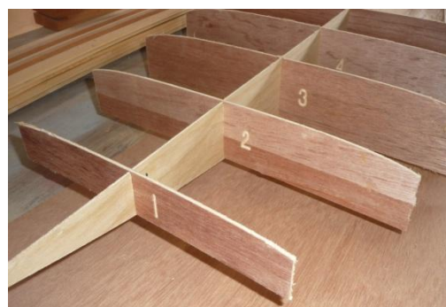
Wood blocks need to be added for the fin box and leash cup. Glue blocks from rib 1 to the back of rib 4.
