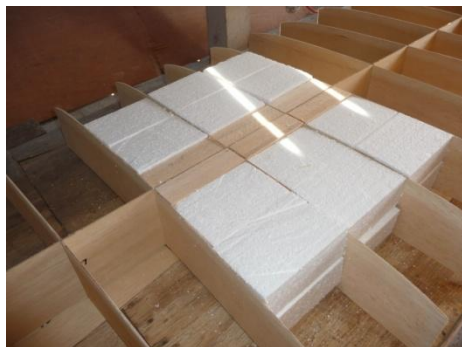
Foam blocks are recommended when sails larger than 7 sq. meters will be used.
