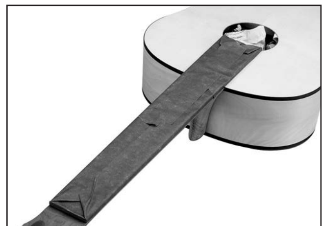
Figure 10. Example of a masked fingerboard and stuffed sound hole.
