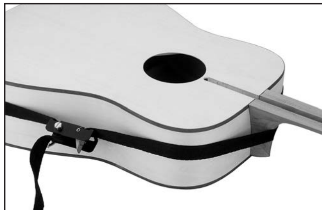
Figure 4. Securing the guitar neck to the body.
