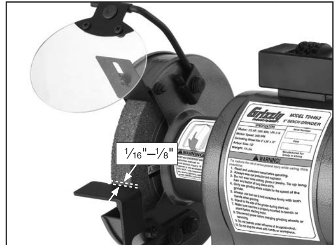
Figure 11. Model T24463 tool rest gap.
