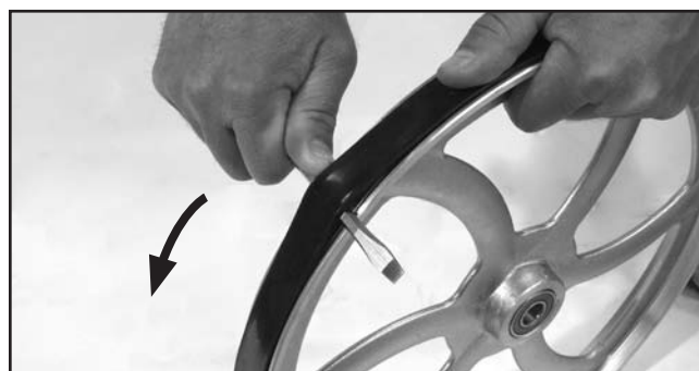
Figure 3. Using a screwdriver to help center the tire on the wheel.
