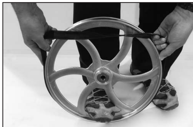
Figure 2. Installing the tire on the wheel.
