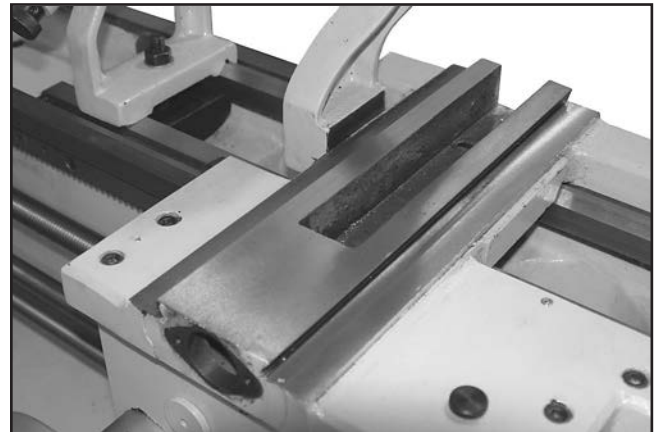
Figure 10. Cross slide removed from saddle.
