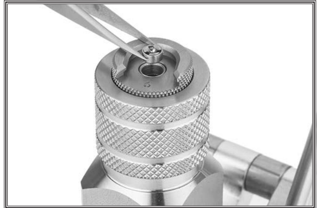
Figure 6. Inserting primer into sleeve.
